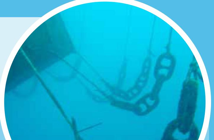
**Description:** Stud link chains used as sinkers. Chains are preferable for use as net tensioning ballasts because greater weight in water of steel, compared with concrete, stones or other materials.
